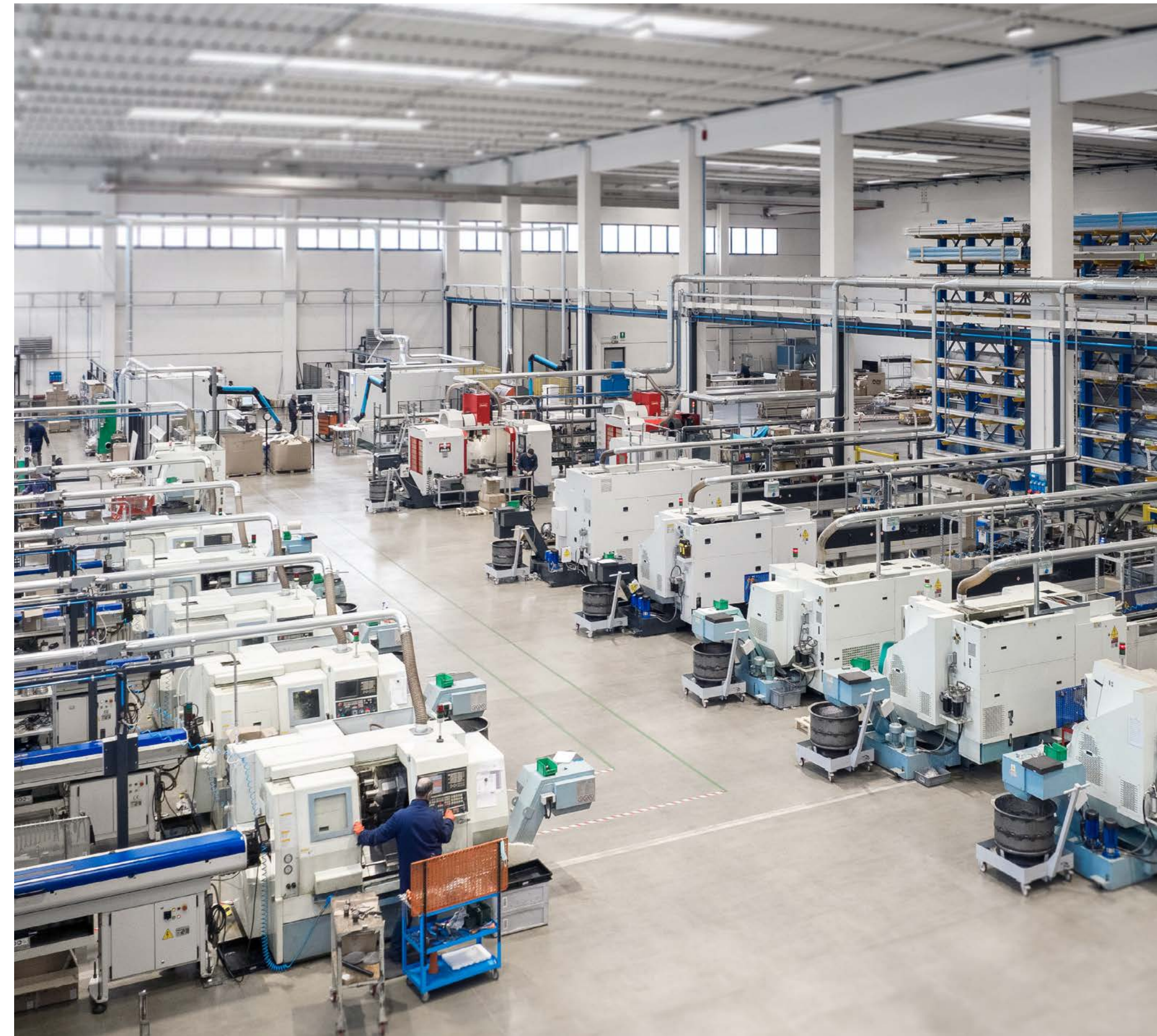
Two cutting lines and 22 CNC machines, with a glimpse of the aluminum semi-finished product storage area, ready for sectioning based on project requirements.
