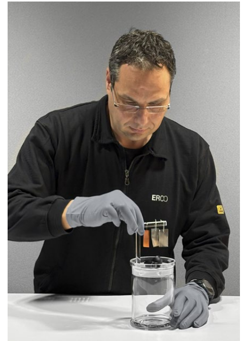
Oddy test with Axis showcase luminaires
